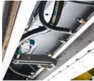
Ice wash system Multijet with suction ledge
