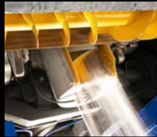
Screw conveyor wash system vertical
