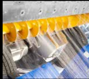
Screw conveyor wash system horizontal
