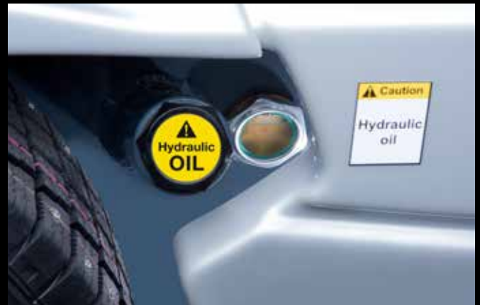
Good sight: Hydraulic oil level indicator
