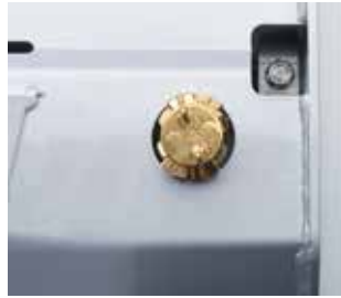
Screw conveyor wash system horizontal
