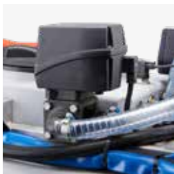
3-way valve, electrically controlled from the monitor (treatment/ flushing)
