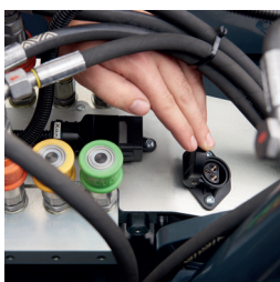
Switchable 12V socket according to DIN 9680
