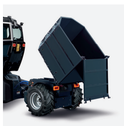
Tilting device with hydraulic actuation
