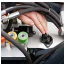
Switchable 12V socket according to DIN 9680
