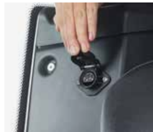
Switchable 12V socket according to DIN 9680
