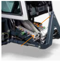
Hydraulic power unit & 12V socket
