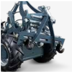
Three-point mounting frame Cat. 1, pivotable ( \pm 15^\circ ) and with side shift
